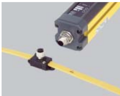
Abb. 5.3-1: Connecting the sensor with an M12 connector socket by means of an M12 bus terminal to AS-Interface
