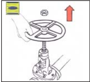
Fig. 1. Ensure valve is in open position and L.O Key can be released before installation. Remove existing valve hand wheel and nut. Discard both.
