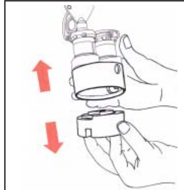
Fig. 3 Separate lock from adaptor and anchor.
